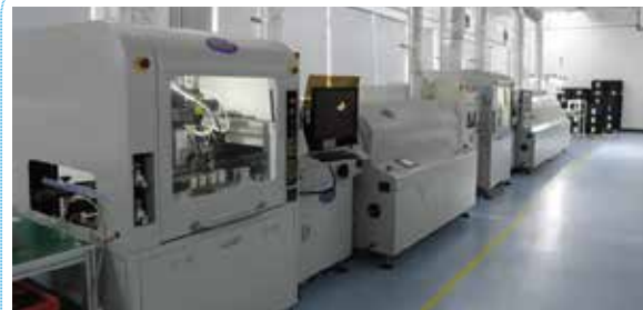
Note: The automatic spraying line of three-proofing lacquer
