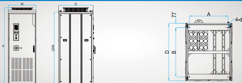
Structural dimensions and installation diagram for C10 cabinet
